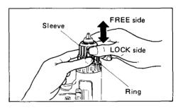
Place the bit in the chuck as far as it will go. Hold the ring firmly and turn the sleeve clockwise to tighten the chuck. Then push the sleeve down toward the "LOCK" side. See illustration.
